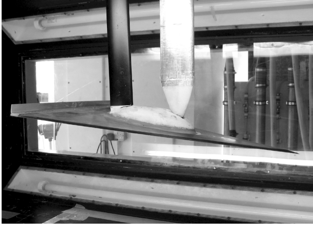
Fig. 3 Model mounted in the Bristol Low-Turbulence Tunnel.
